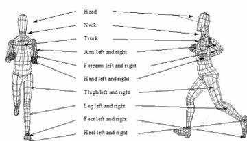
Figure 1: MAN3D human model representation and its 17 segments.
