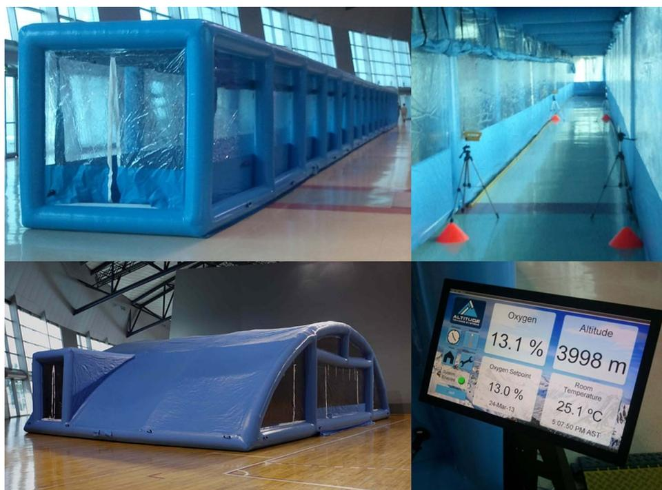
**Figure 1** The mobile inflatable simulated hypoxic equipment as it was presented during the Doha conference. External (top left panel) and inside (top right panel) tunnel views are pictured along with the rectangular design (bottom left panel) and touch screen controller (bottom right panel).
